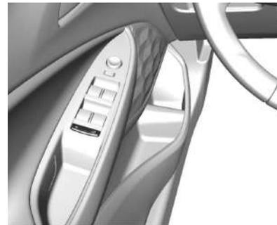
Pulse el interruptor
